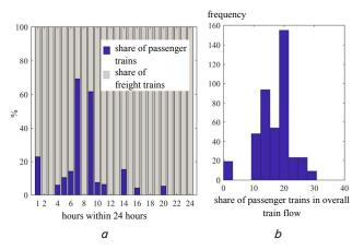
Fig. 4. Dependence of the number of passenger trains on the overall train flow at the section Osnova-Lyubotyn: a - dynamics of change in the share of passenger traffic within the overall train flow over 24 hours; b - dependence of frequency on the percent share of passenger traffic on average over 24 hours
