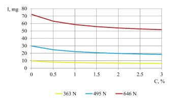
Fig. 2. Change in the amount of roller wear  $R_1$  depending on the concentration of graphite powder in the industrial oil I-12A under different external loads
