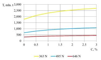
Fig. 4. Resource of a rail depending on the concentration of graphite powder in the industrial oil I-12A under different external loads
