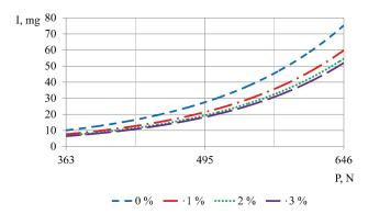
Fig. 3. Change in the amount of roller wear  $R_1$  depending on the external load at different concentrations of graphite powder in oil I-12A
