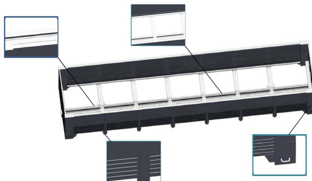
Fig. 6. Finite-element model of the body of a gondola car
