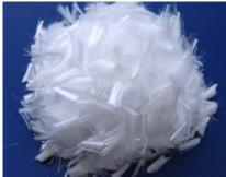
**Fig.6 Polypropylene fibrous**
