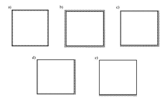
Fig.3 Schemes of supporting slabs: a) with hinge-supported edges; b) with fixed edges;
