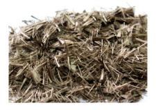
**Fig.5 Basalt fibrous**
