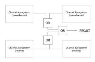
Pic.4 The structural scheme of realisation service functions.
