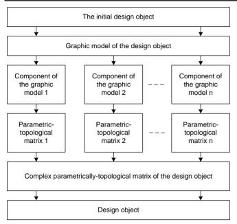
Fig.1. Scheme of graphical-analytical design
