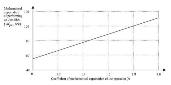
Fig. 3. Mathematical expectation  $M_{pe}$  of execution of the operation of moving the point with false clear of the track area.
