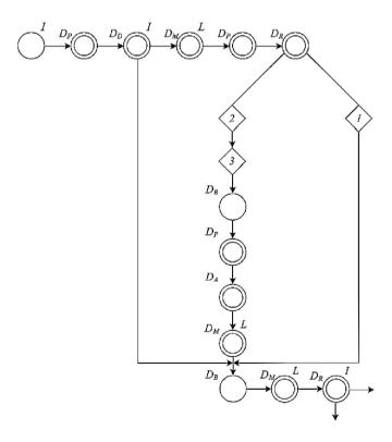
Fig. 2. Functional-semantic network of the performance of the DSP operation when moving the point with false clear of the track area.
