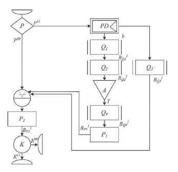
Fig. 1. Functional-semantic network of the performance of the DSP operation when moving the point with false clear of the track area.
