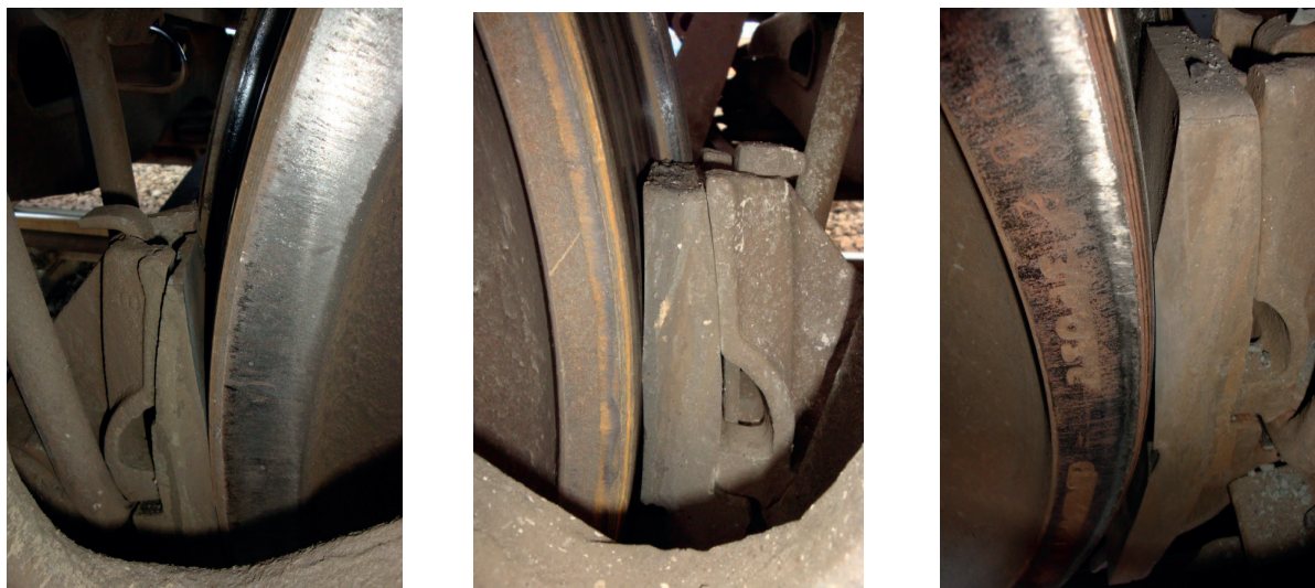
Figure 1 Wagon pads with wedge-dual wear
