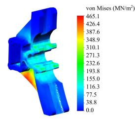
Fig. 11. The stressed state of the shoe
