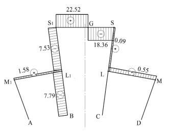
Fig. 8. Diagram of shear forces QX
