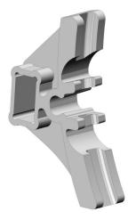
Fig. 9. Spatial model of the brake shoe
