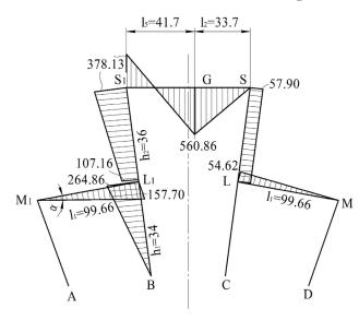
Fig. 7. Estimation diagram of bending moments MX
