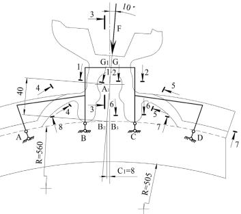
Fig. 2. Shoe-to-pad load transfer diagram (mm)
