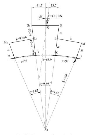
Fig. 3. Estimated shoe diagram (mm)
