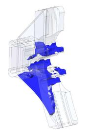
Fig. 12. Zones of the greatest load on the brake shoe
