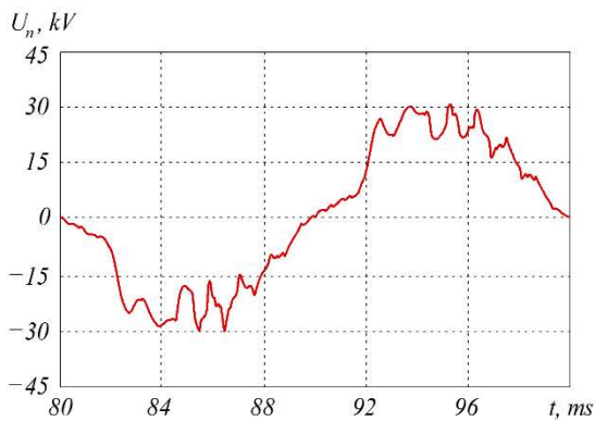
Figure 3. Diagram of the voltage in the contact network with the proposed algorithms of the rectifier-inverter converter
