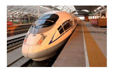
CNR's latest high-speed train CRH380B (pictured) has a design speed of 400 km/h, an operating speed of 350 km/h, and a maximum output of 18.4 MW with half the cars powered. The train has improved aerodynamics by enclosing the inter-car bellows with rubber sections and enclosing the bogies more than on CRH3.
