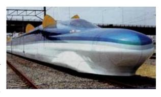
brakes for emergency halt protruding<sup>7</sup> from the roof. In Japan the train got a nickname 'cat-eared Shinkansen'. FASTECH 360 trains will have an arrow-line shape with a 'duck-bill nose'. Like most high-speed trains, FASTECH 360 will have distributed traction instead of power cars. The modular concept implies grouping cars in two three-car sections linked together with a so-called key car. Production trains are expected to enter service in 2011.
