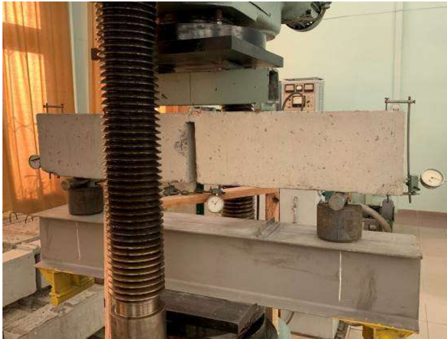
Figure 1 – General view of the experimental installation with location of indicators
