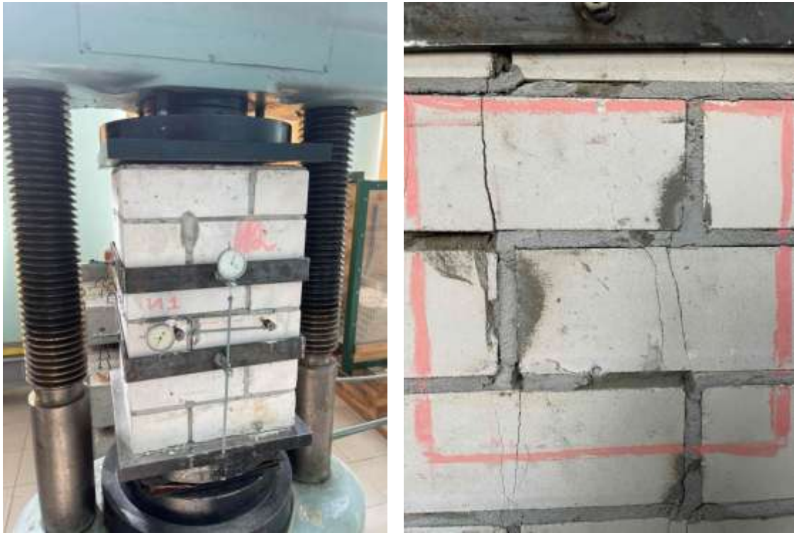
Figure 1 – General view of the experimental installation, the disposition of cracks formation and their density
