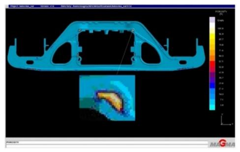
**Fig. 4.**The distribution of internal casting defects in the longitudinal section of chassis side frame 18-100, determined in MAGMA software.
