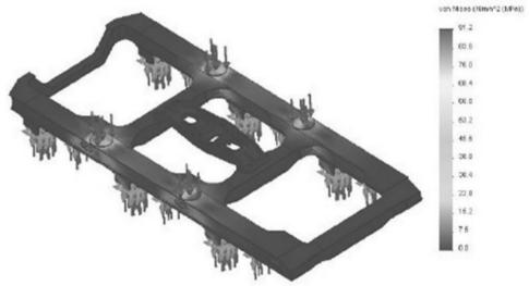
Fig. 6. Results of calculation of stress values in the frame of the diesel locomotive chassis under static loading in the SolidWorksSimulation software package.
