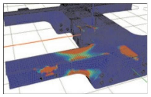
Fig. 7.Results of calculating the longevity of the locomotive chassis frame in the "Universal Mechanism" PC.
