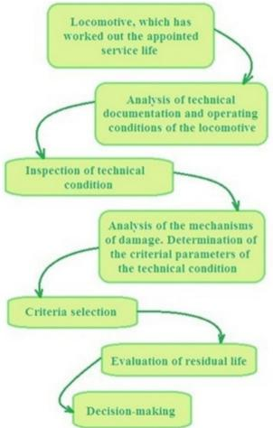
Fig. 1. Block diagram of the procedure for determining the remaining service life extension.
