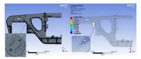
**Fig. 5.**The finite element grid at the top of the crack (a) and the results of calculating KI (b) from the effect of the vertical load on the side frame 18-100.
